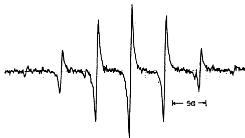
Fig. 3. ESR spectrum of trineopentylgermyl radical at -60^{\circ}\text{C} .
